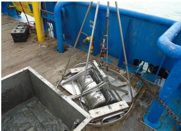
Photo 15 Collection of sediment from Reference area utilizing double van Veen sampler.
