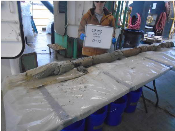
Photo 9 View of sediment collected during DMMU-07C resampling.
