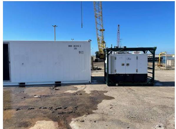
Photo 14 View of refrigerated unit at Martin Energy facility used to store samples at or below 4°C following collection.
