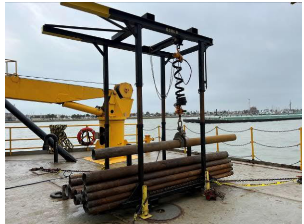
Photo 4 View of sonic drilling rods.
