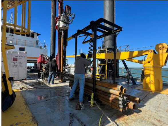
Photo 1 Advancement of boring CDP-06A utilizing sonic drill rig during 2023 resampling event.
