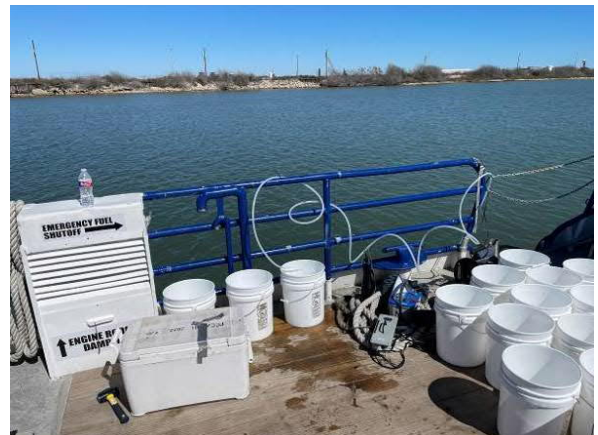
Photo 18 Typical set-up used for collection of marine water from DMMUs specified in SAP.
