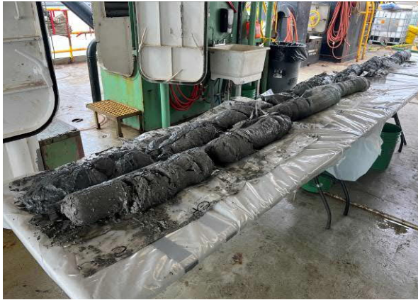
Photo 7 View of sediment collected during DMMU-07A resampling.
